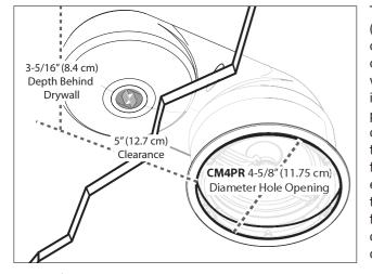
Figure 1. CM4PR loudspeaker installation dimensions
